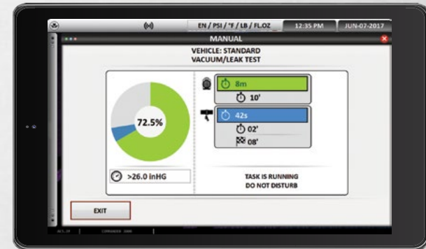
Vacuum/Leak Test Screen fully customizable options allows the user to personalize the times of vacuum and leak testing
