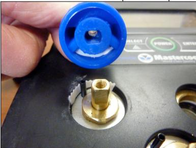
The orientation of each knob must be such that the black rolled pin fits inside the white region of each knob. The white region is only shown in the picture for clarification. After the knobs are positioned as instructed, tighten them with the screws previously removed in Step #1. Check to verify that each now rotates only
