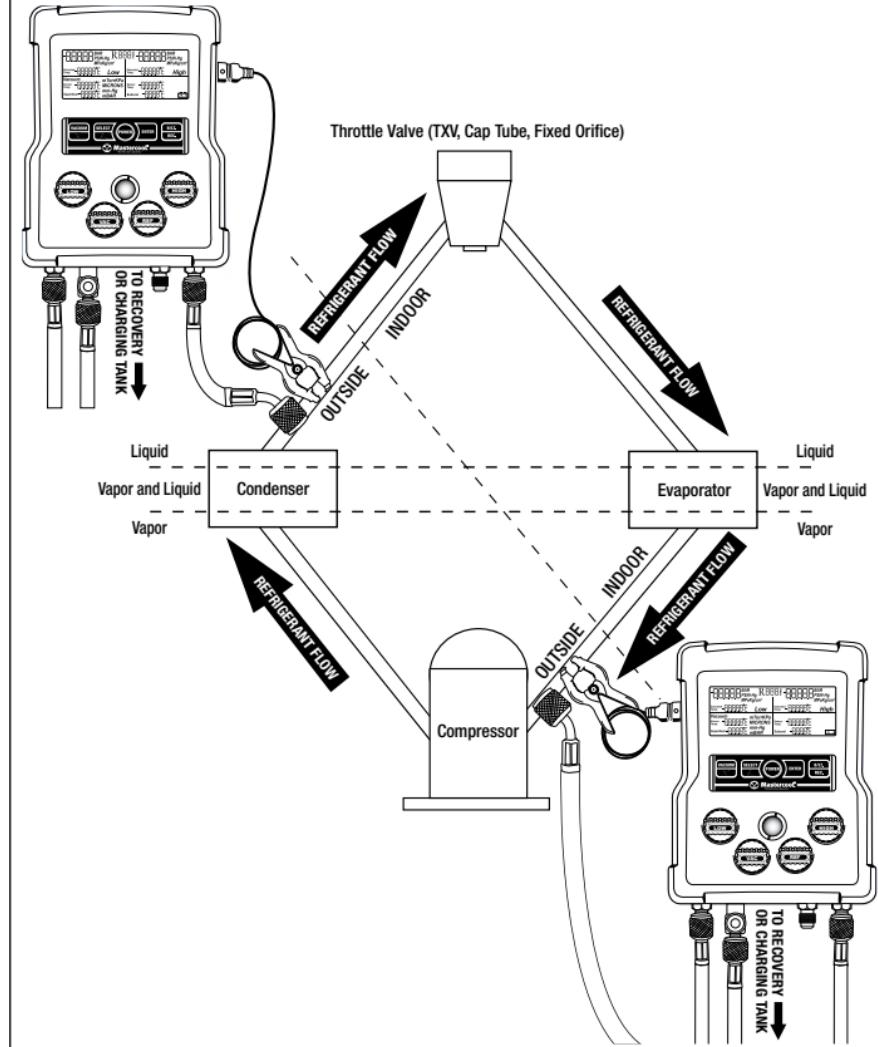
On TXV systems, the subcooling is the best indication of the state of the charge in the refrigerant system since these systems are designed to maintain constant superheat. Properly charging a system ensures maximum efficiency and longer equipment life.
