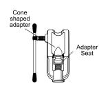
9) Loosen the tightening bar and remove the tube. It should look something like the sketch below.
