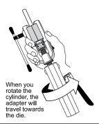
5) Begin squeezing the lever and continue until the edge of the adapter meets the die or pumping action shows substantial resistance.
