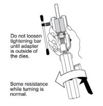
6) Release the pressure by opening the relief valve.
