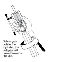
Begin squeezing the lever and continue until the edge of the adapter meets the die or pumping action shows substantial resistance.
