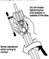
8) Loosen the tightening bar and remove the tube. It should look something like the sketch below.
