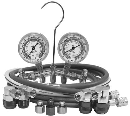
service hose (red) to the discharge side of the compressor. Make sure the couplers are securely snapped.
