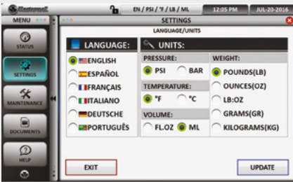
Settings Screen allows the user to select a default language, units, temperature, volume and weight measurement
