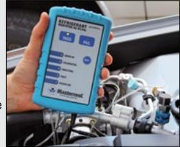
**691234YF-MINI MINI ID, IDENTIFICATEUR DE RÉFRIGÉRANT POUR R1234yf**
