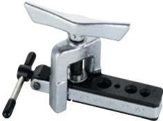
Sliding Die-Block 45° Flaring Tool Flares and Burnishes 6 Sizes: 3/16, 1/4, 5/16, 3/8, 1/2 and 5/8" O.D. Tubing.
