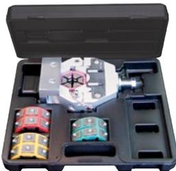
The 71550 is our "manual style" A/C hose crimper. The dies snap quickly into place requiring no pins or screws. The unit can be easily mounted to a bench using the holding fixture or held securely in a vice. This kit comes with a complete set of dies covering standard hose sizes #6, #8, #10 and #12. **PATENT# 6,324,884**
