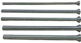
Economical and effective tools for bending soft copper or aluminum tubing without kinks. Special nickel plated, spring steel is flared on one end for quick tube insertion. Each tool bends one size.
