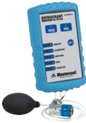
The Refrigerant Identifier helps confirm the presence and quality of R134a refrigerant in vehicle air conditioning systems.
