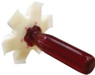
Cleans and straightens condenser and evaporator fins. Six sided head for 8, 9, 10, 12, 14 and 15 fins per inch applications.
