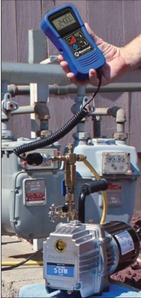
As a professional technician the assurance of a deep vacuum on a system is imperative. The main problem with many small handheld units is their inaccuracy and durability. Although the thermocouple sensor has been proven to be much more accurate and durable than the thermister type, the problem has been the inconvenience of a cumbersome tabletop unit.
