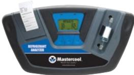
The Ultima ID Pro2 HVAC/R Refrigerant Analyzer enables fast, accurate testing of refrigerant, reducing the need for costly and time-consuming gas chromatography.
