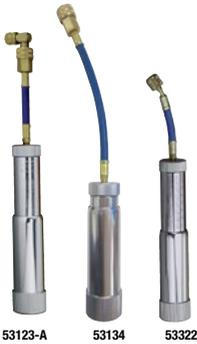
To inject the oil or dye, simply connect the injector to the low side of the A/C system and twist the handle until you reach the desired amount.
