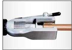
The copper tube is secured in the holding fixture by the forming dies. The hydraulic pump pushes in the forming adapter to fabricate the flare or swage. This cut-away photo shows the forming process.
