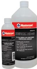
ZEROL HD46 is a fully formulated ISO VG46 grade polyalkylene glycol lubricant designed specifically for application with HFO refrigerant R1234yf in mobile air conditioning (MAC) systems. The product is a double end-capped PAG, and is manufactured to exacting standards of high double endcapping efficiency. ZEROL HD46 is suitable for use in both belt and electrically driven compressors utilizing R1234yf, and is also fully suitable for use in R134a belt-driven and electric MAC compressors.
