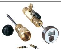
Special valve core remover/installer adapter allows replacement of damaged or faulty service valve cores without recharging the system. Valve replacement no longer requires time consuming refrigerant recovery. Calculation of superheat with excellent accuracy by reading refrigerant temperature and pressure from the same location in the system.
