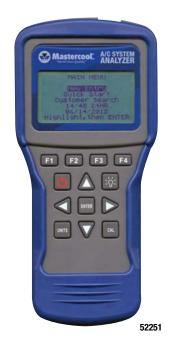
Mastercool's new A/C System Analyzer is an all-in one tool that not only calculates critical information for the air conditioning system but also diagnoses basic system problems. The LCDdisplay leads the technician through basic tests making service quicker and less complicated. The A/C System Analyzer is able to calculate: Actual Superheat, Subcool, Target Superheat, Temperature Split, Dry Bulb, Wet Bulb, Relative Humidity, Dew Point, Air Velocity and Air Flow Volume.
