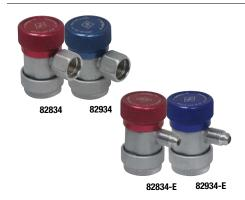
Patented manual couplers adjust easily to R134a service ports with varying dimensions. All metal construction for extra durability. Patented, spring loaded depressor will not damage service valves. Can be removed from service ports regardless of knob position without losing refrigerant. Meets SAE, UL and EPA requirements for containment of refrigerant. Color coded. **PATENT# 5,370,359**
