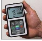
When remote is out of range the unit will automatically pause. This pause mechanism allows unit to restart when remote is back in range.
