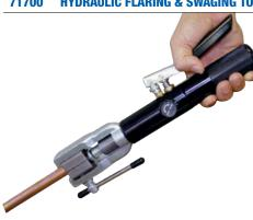
This kit features a hand-held hydraulic press that accurately flares & swages copper tubing. Once the die and adapter are secured in the fixture, a few pumps of the handle and you're done! This tool really takes the work out of swaging and flaring, especially on larger tube sizes. The kit includes dies and adapters for flaring and swaging copper tubing sizes 1/4, 5/16, 3/8, 1/2, 5/8, 3/4 and 7/8." Comes in custom molded carrying case. PATENT# 5,782,128
