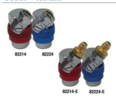
This unique patented design easily snaps on and off the A/C systems service ports under any pressure. The E-Z Snap™ automatically adjusts to various service port dimensions allowing fast and immediate access into the A/C system. The swivel feature enables the user to easily access all service ports, even in the tightest quarters. Meets SAE, UL, and EPA requirements for containment of refrigerant. **PATENT# 5,244,010**
