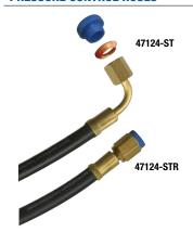
Replaces regular copper capillary tubing and eliminates capillary failure due to work hardening from vibration.
